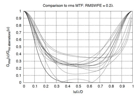
Figure 2: The rms MTF for an unobstructed aperture with aberrations, relative to the unaberrated case at RMSWFE =  $0.2\lambda$ . The solid curve is the fitting formula used in the ETC. The dashed curves are low-order aberrations. There are 13 cases shown, with different aberrations: defocus, astigmatism, coma, and trefoil; and cases with 25:75, 50:50, and 75:25 mixtures of defocus with the other three aberrations.
