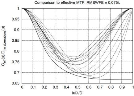
Figure 1: The effective MTF for an unobstructed aperture with aberrations, relative to the unaberrated case, at RMSWFE =  $0.075\lambda$ . The solid curve is the fitting formula used in the ETC. The dashed curves are low-order aberrations. There are 13 cases shown, with different
