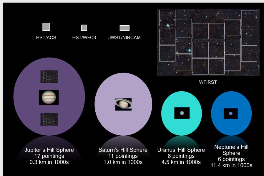
**Above:** WFIRST/WFI FOV compared to the FOVs of other instruments on HST and JWST. Each of the 18 individual white boxes represents one detector in the WFI FOV. The WFI can cover the entirety of the giant planet Hill spheres in 6-17 separate pointings to observe irregular satellites.
