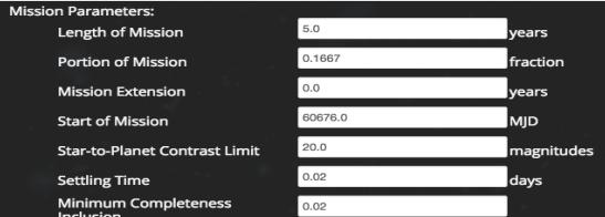
Screenshot of part of the EXOSIMS (Delacroix et al. 2016; see also posters 246.04 and 246.06) input GUI at ISOC. The user specifies input parameters, and the results are returned both as graphical output and a downloadable table.
