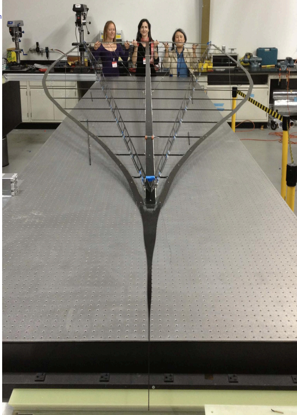
Petal prototype used for manufacturing tolerance verification tests. Credit: NASA/JPL
