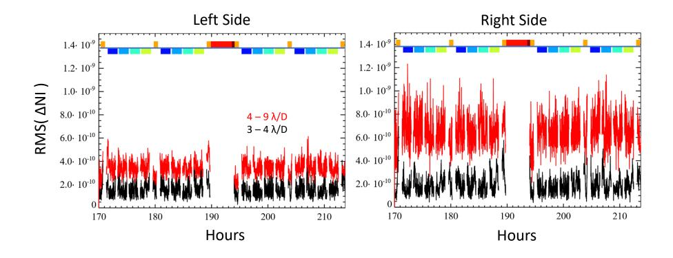
The high-frequency noise is due to imperfect LOWFS measurement and correction (the LOWFS was tuned for worse stability). The noise averages out over time.
