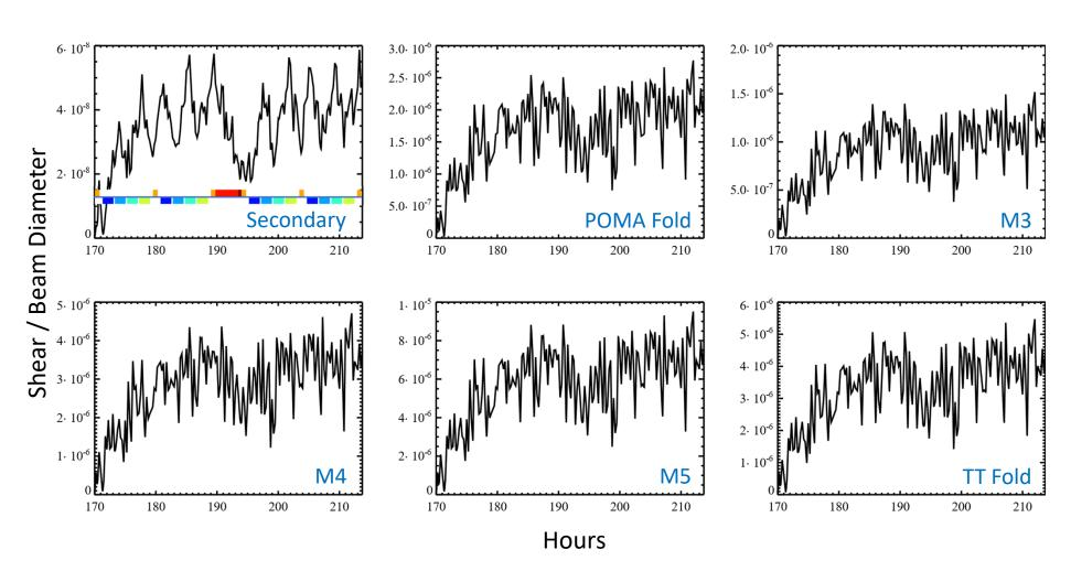
CGI bulk shear (X,Y displacement at FSM relative to instrument carrier)
