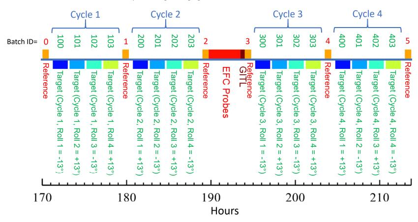
EFC Probes: apply pre-defined DM patterns & record resulting image changes; no images are provided for this span GITL: Download probe images to ground, use them to derive wavefront error, compute new DM solutions, upload them to CGI
