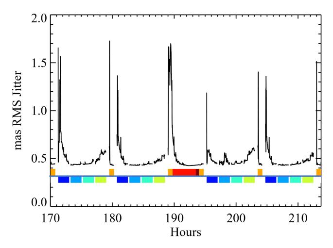
The jitter floor here is set by a 0.3 mas RMS (per axis) system noise that is RSSed with the predicted post-steering-mirror jitter.
