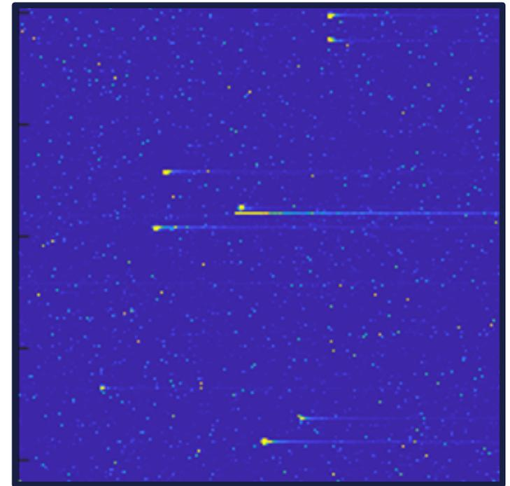
Ground EMCCD test data showing muon cosmic rays against a backdrop of dark current
