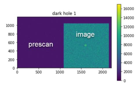
The clocking of this serial register occasionally creates ``clock-induced charge'' (CIC), at a rate much less than 1 electron per pixel per frame. These CIC electrons go through the gain register and result in an EM amplified signal. Since the EM gain process has a distinct probability distribution function (Basden 2003), fitting a histogram of the observed serial prescan CIC counts to the known distribution can provide both the EM gain and the average CIC rate.
